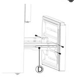
4. Remove the 4 screws attached to the supporting frame (D).
